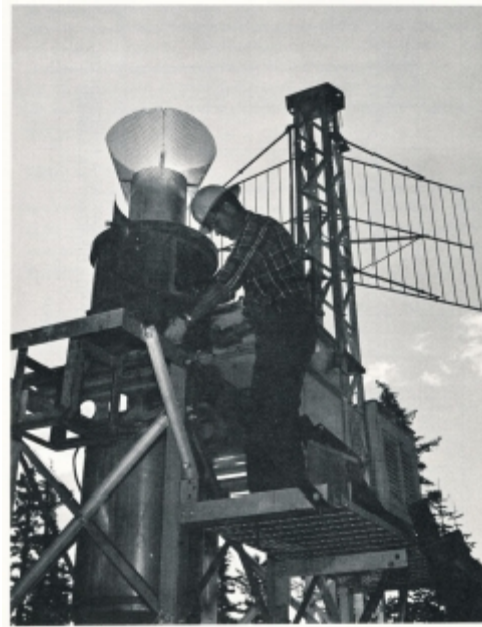
Fig. 17 -- Pacific Gas & Electric Company ground-based silver iodide generator.
