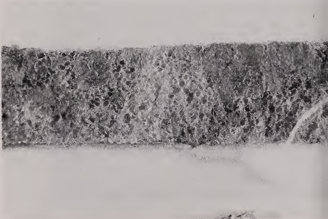
Strip of seat padding showing reddish residue from missile exhaust.
