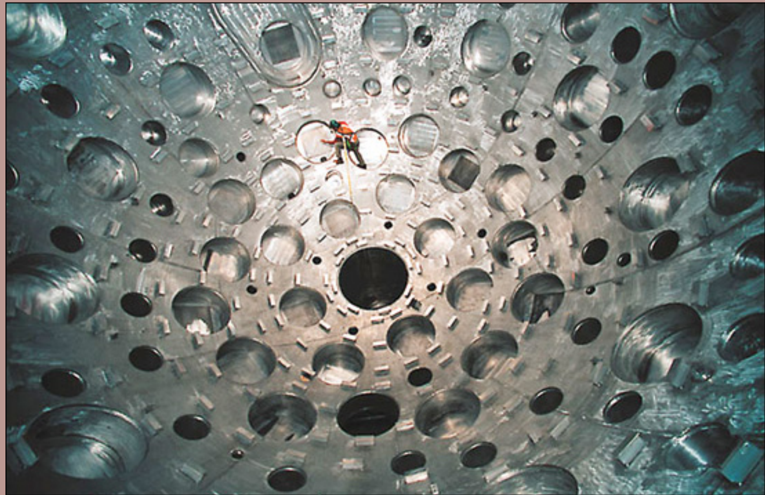
employee (top center), working inside a fusion reactor chamber
