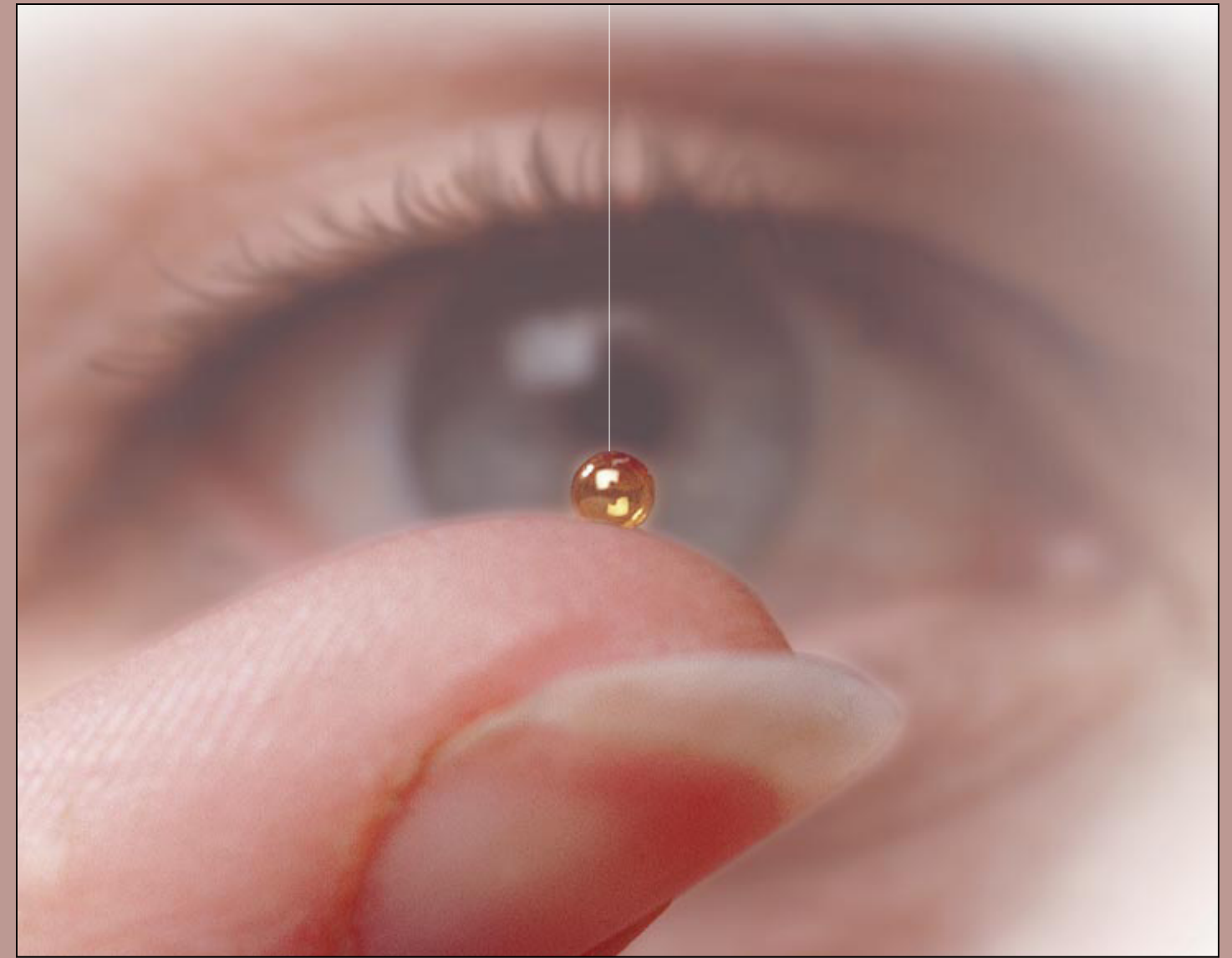
NIF's fuel "target", filled with either Deuterium-Tritium gas or D-T ice. The capsule is held in the hohlraum using thin plastic webbing. A ten micrometer filling tube is barely visible extending upwards from the top of the capsule.
