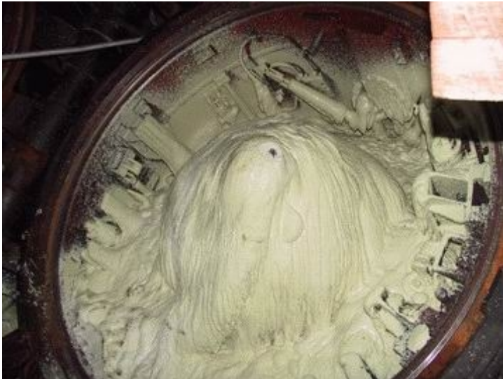
Above – rare photograph of one of the “Kursk’s” missile silos filled with foam.
