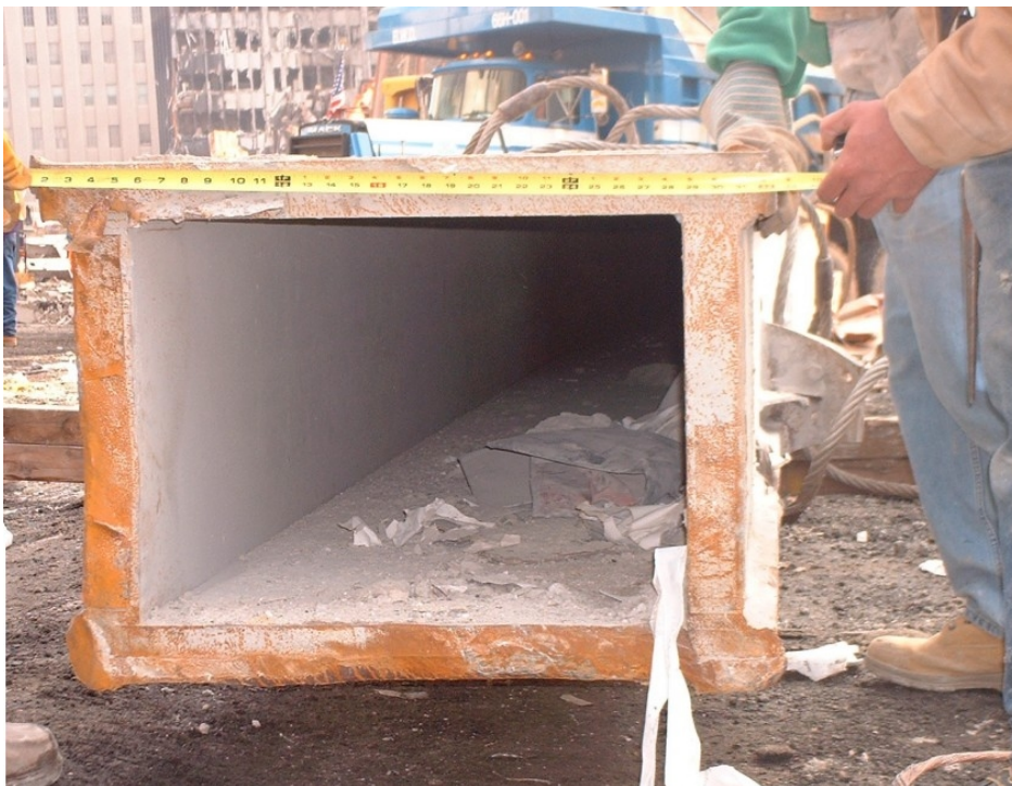
It is good to look at these Twin Towers' perimeter columns again and realize, at last, that their thick walls were more than comparable with armor used to make main-battle tanks. To penetrate such a column
