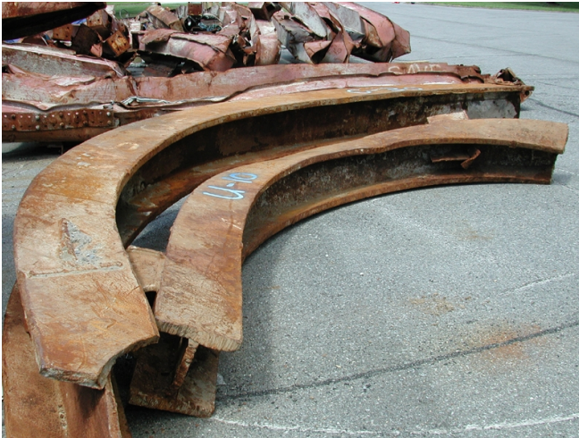
Above – an H-type 2.5 inch thick steel perimeter column of the upper parts of the WTC Twin Tower found at ground zero (the thickness of its main walls is the same as the thickness of the column on the above picture).
