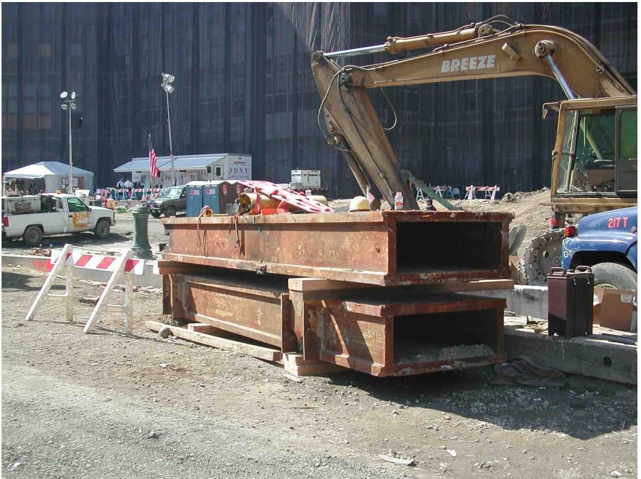
Above – typical WTC perimeter columns at “ground zero” on October 3, 2001.
