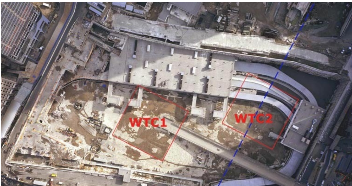
Above – an aerial photograph of the actual “bathtub” showing PATH tunnels during the PATH station construction. Below – a graphic representation of the bathtub area damage sustained as a result of the WTC collapse and its description from the New York Times.
