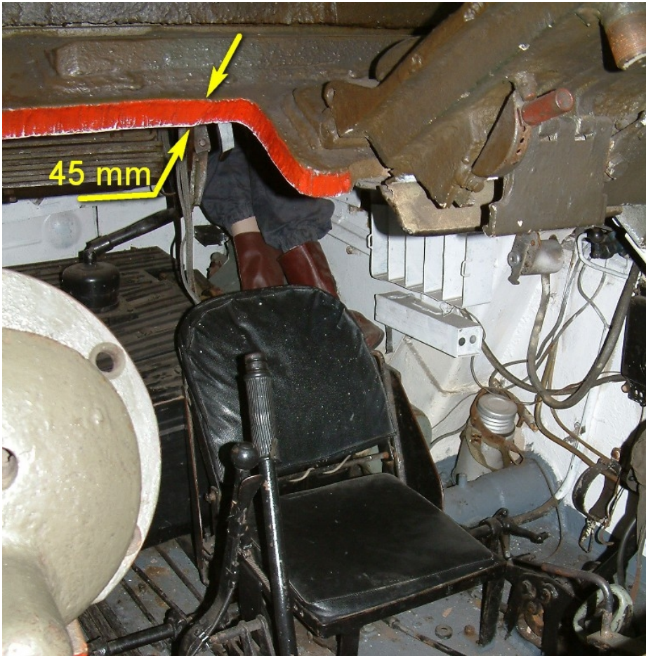
Above – a driver's compartment of the T-34 tank showing the driver's seat and gears through an open hatch and through an additional hole cut in the front armor. The thickness of the cut armor is painted in red. Below – a typical steel perimeter column of the upper parts of the WTC Twin Tower found at ground zero.
