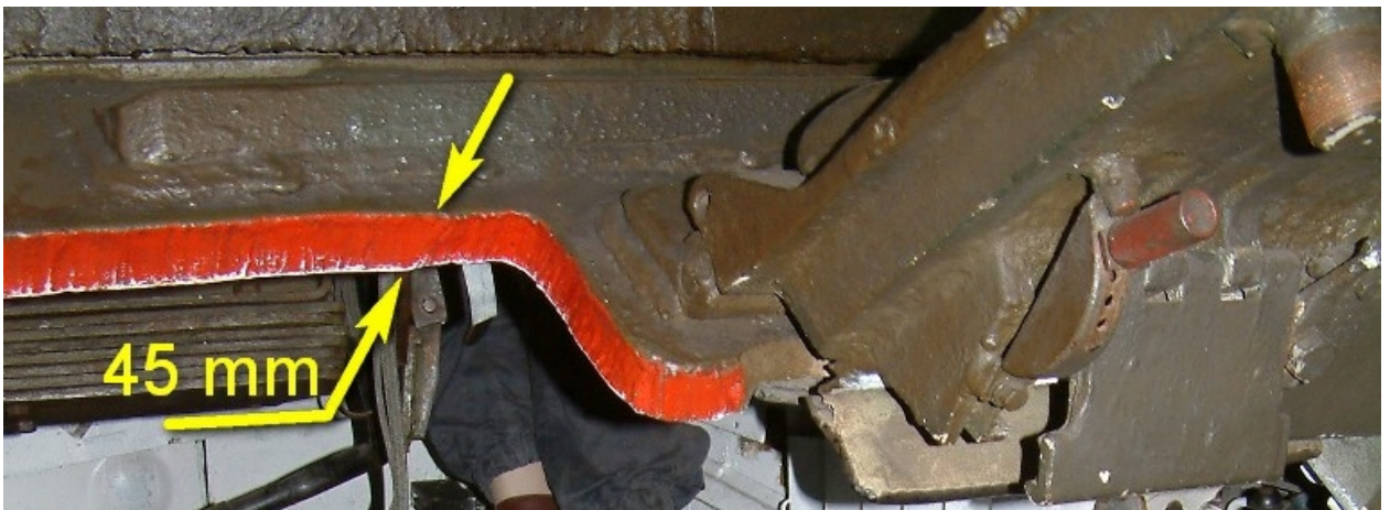
On the photo above is shown the thickness of the T-34 tank’s armor, in case you forgot it.
