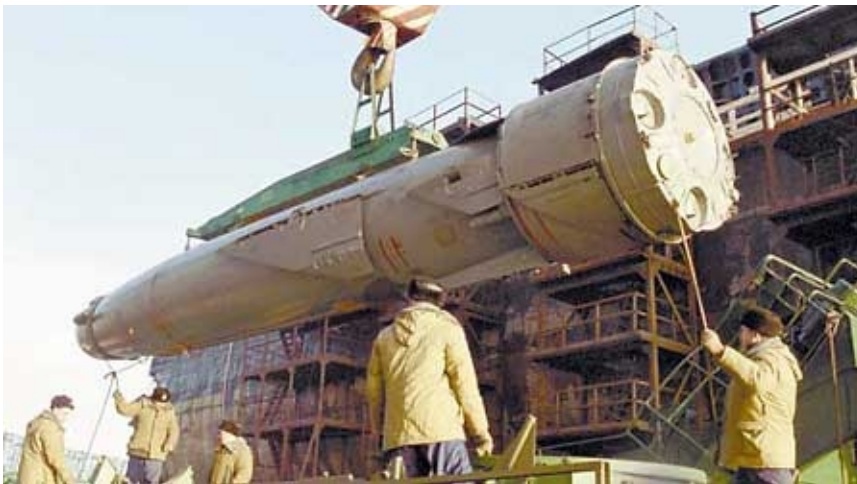
Above – one of such pictures (widely circulated over various mass-media) shows a launch-container with fast-setting foam inside cut from the “Kursk’s” body.
