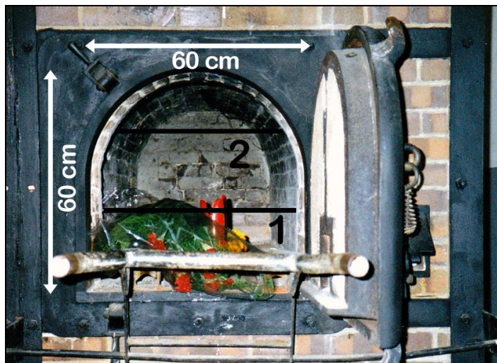
Illustration 36: Coke-fired double-muffle furnace by the Topf Company in the Mauthausen Concentration Camp with identical muffles to those that were installed in Auschwitz. The two horizontal lines represent the height of two corpses on top of each other on the muffle grate (Mattogno 2015, p. 721).
