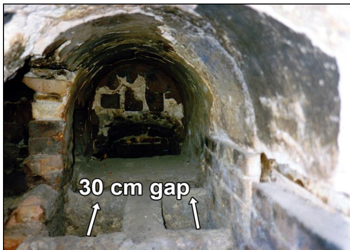
Illustration 38: Interior of the muffle of the Topf Company furnace, Type Gusen, with gaps of 11.81 inch (length) and 9.84 inch (width) in the fireclay grate.
