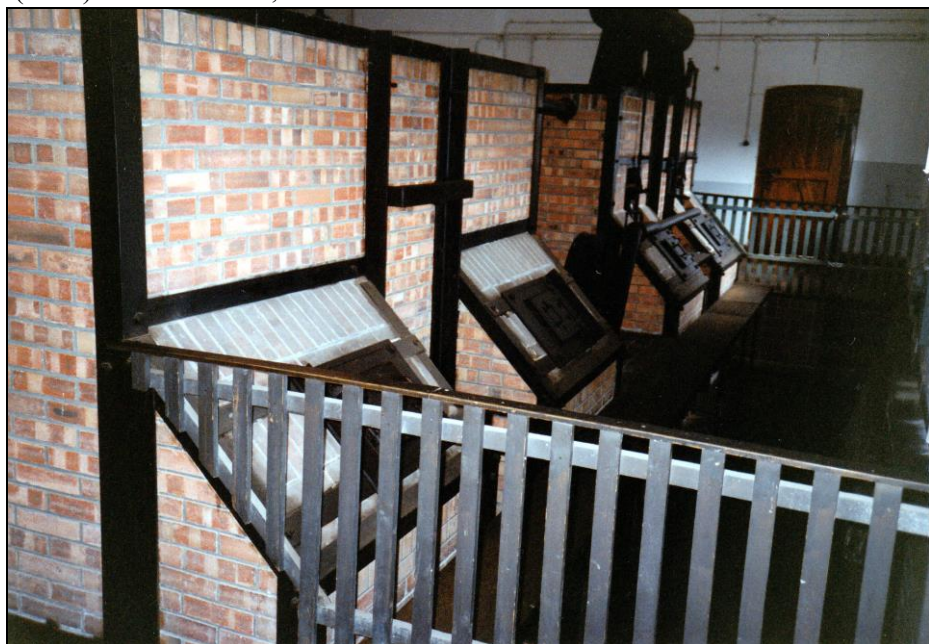
DOCUMENT 12: Gasifiers at the rear end of the two Topf triple-muffle cremation furnaces in the crematorium at the Buchenwald Camp. From: Mattogno/Deana 2015, Vol. III, Photo 205, p. 131.
