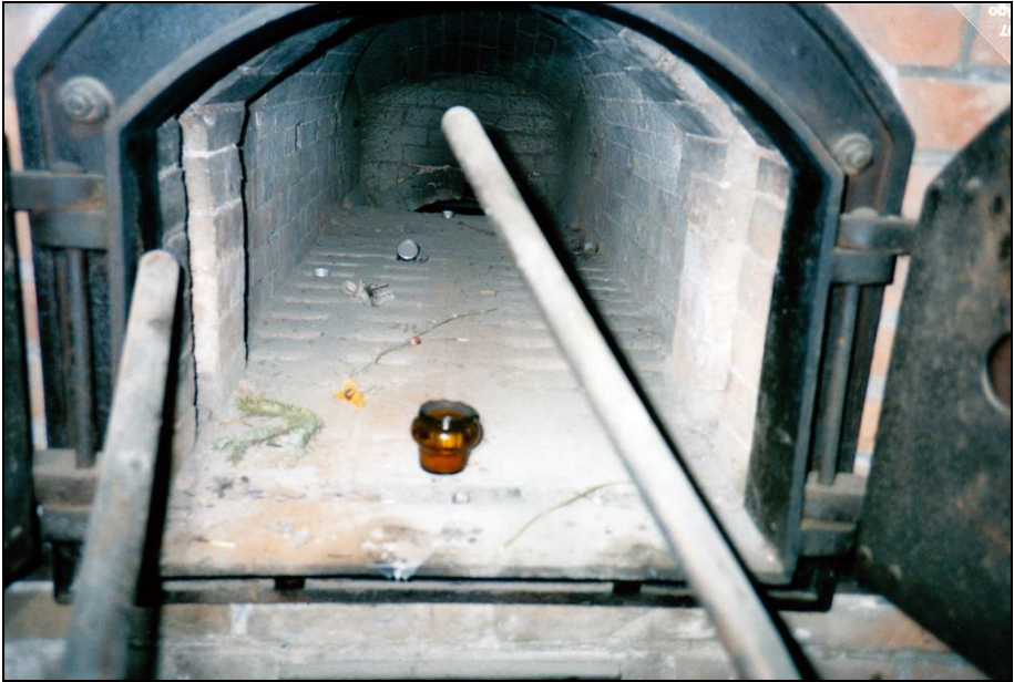
Photograph 296: The center furnace, close-up of the muffle.
