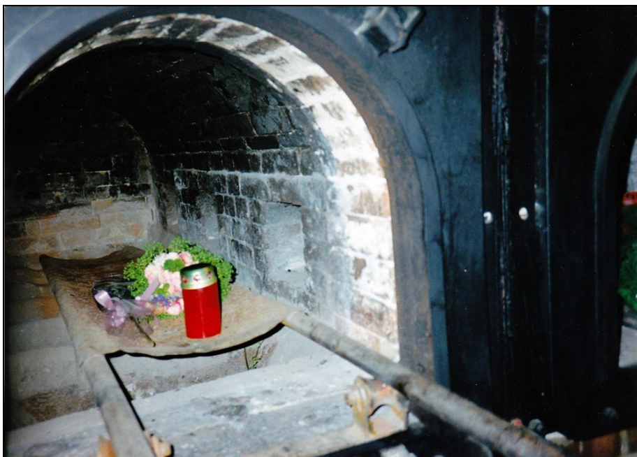
Photograph 63: Left-hand muffle; the three inter-muffle openings can be seen to the right.
