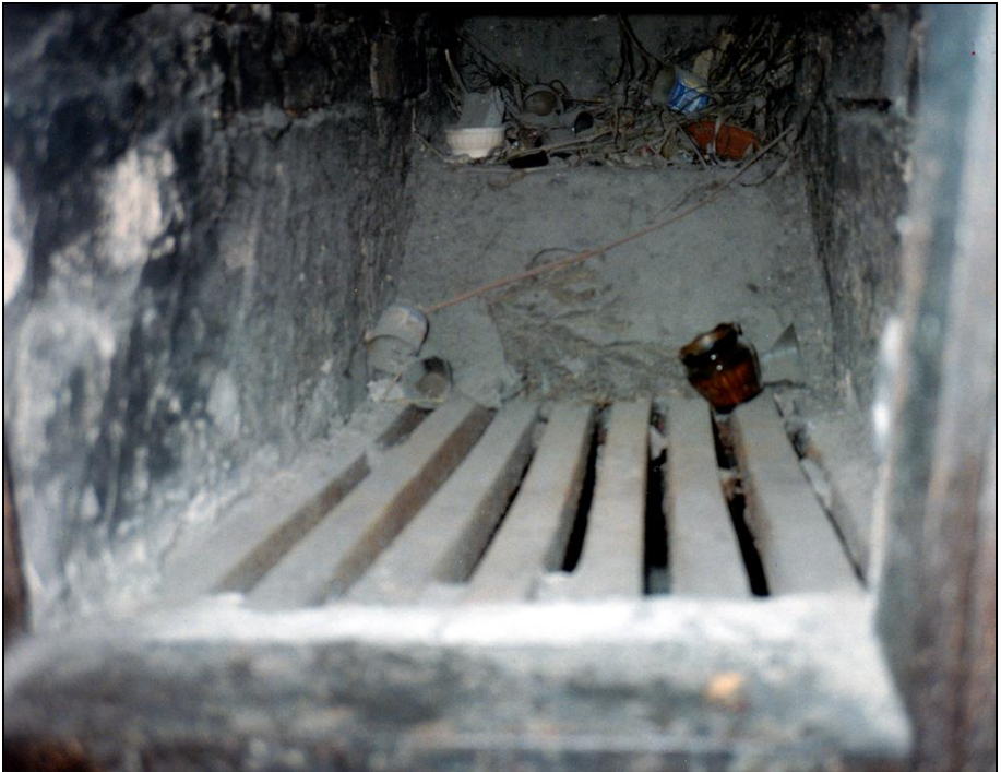
Photograph 99: Furnace 2: original gasifier grate with seven longitudinal bars and two transverse bars.
