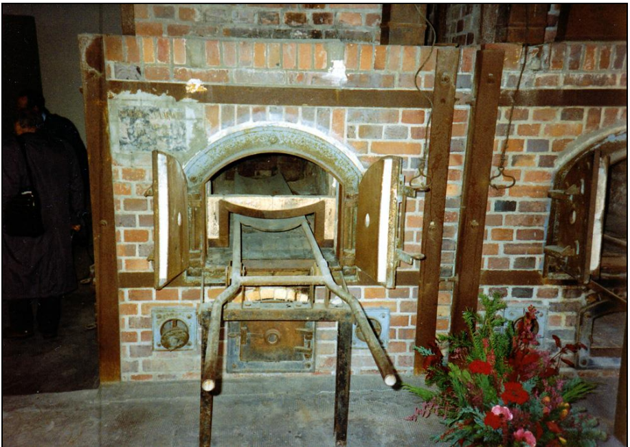
Photograph 265: Second furnace, front view. Muffle with stretcher and lowered corpse-retaining plate made of fireclay.
