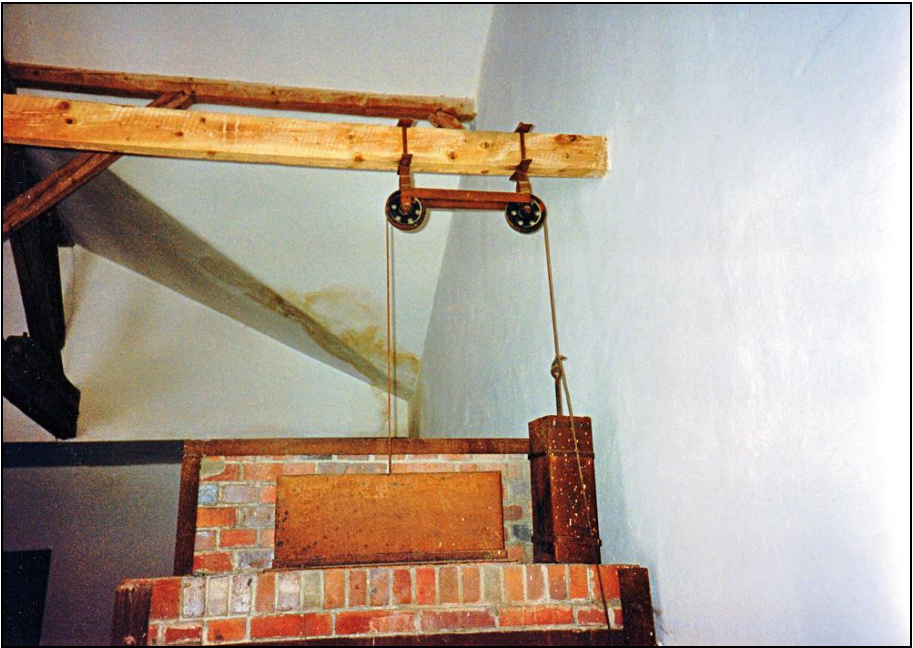
Photograph 255: Fourth furnace, front view: metal housing of the muffle door's corpse-retaining plate made of refractory clay; wire rope, pulley and counterweight for its operation.
