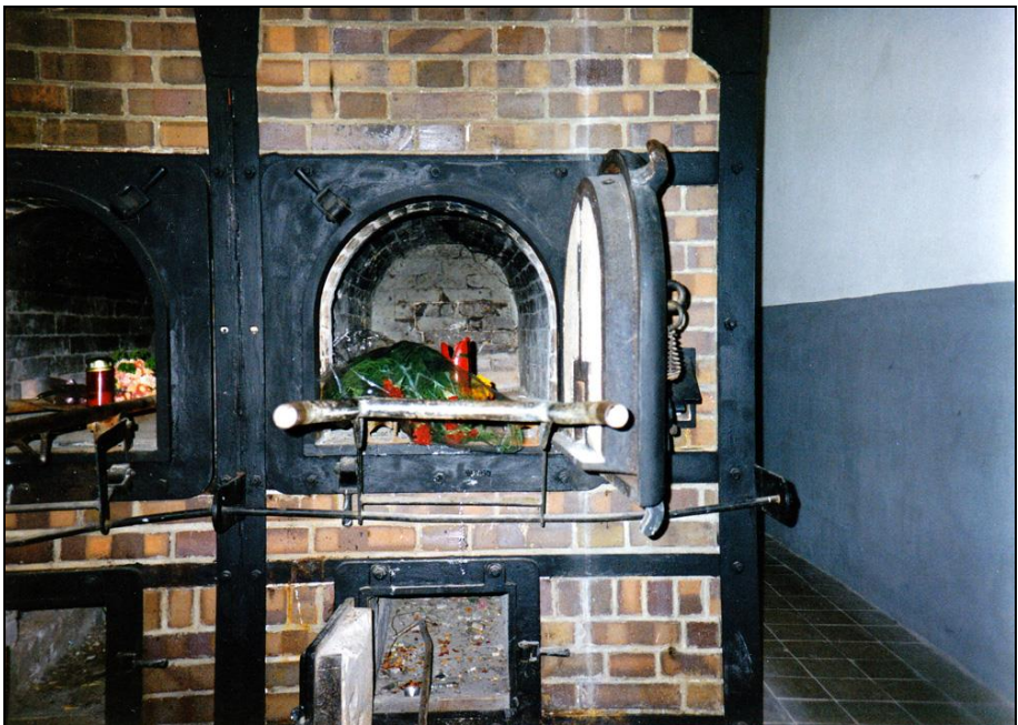
Photograph 83: Loading system of the right-hand muffle: rod mounted to the frame, movable roller device, and stretcher for the corpse.
