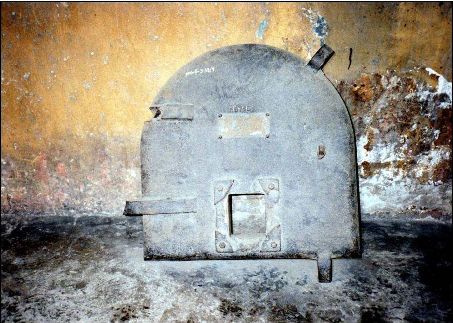
Photograph 128: Muffle door from a TOPF triple-muffle cremation furnace previously installed in either Crematorium II or III at Birkenau.
