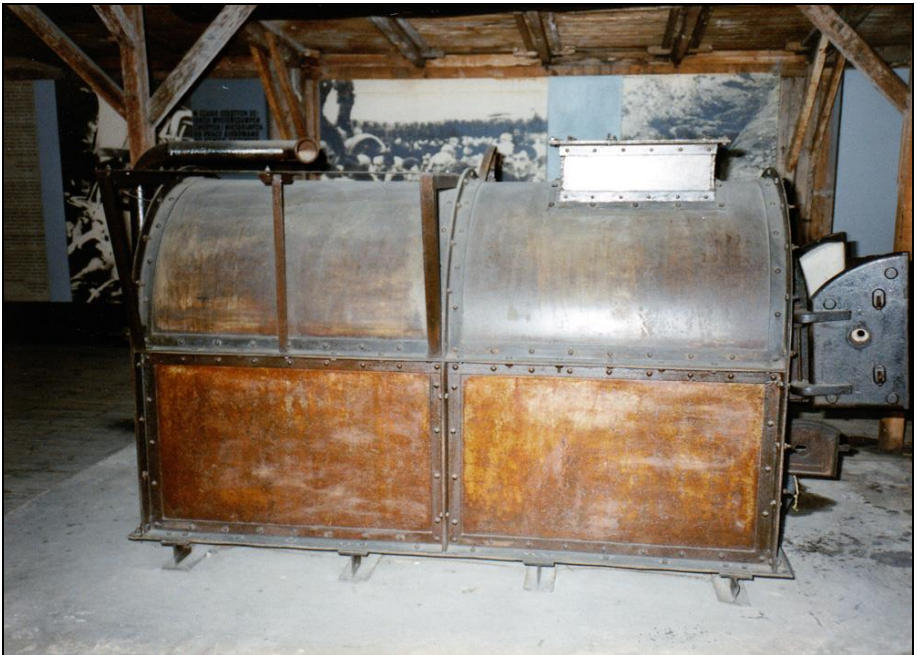
Photograph 325: as above. In the upper part of the furnace can be seen the combustion-air pipe for the burners (left), the support bars for the fan and its motor (center), and the base of the chimney (right).
