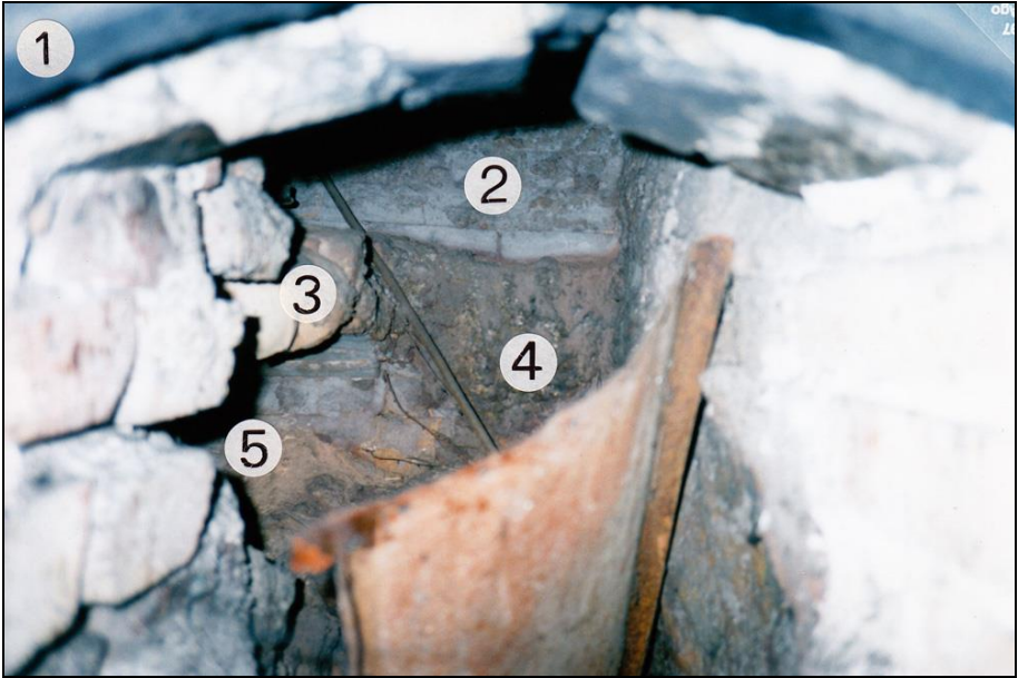
Photograph 278: as above, seen through the coke-loading door. 1: door frame; 2: muffle; 3: muffle grate; 4: gasifier pit; 5: ash chamber.
