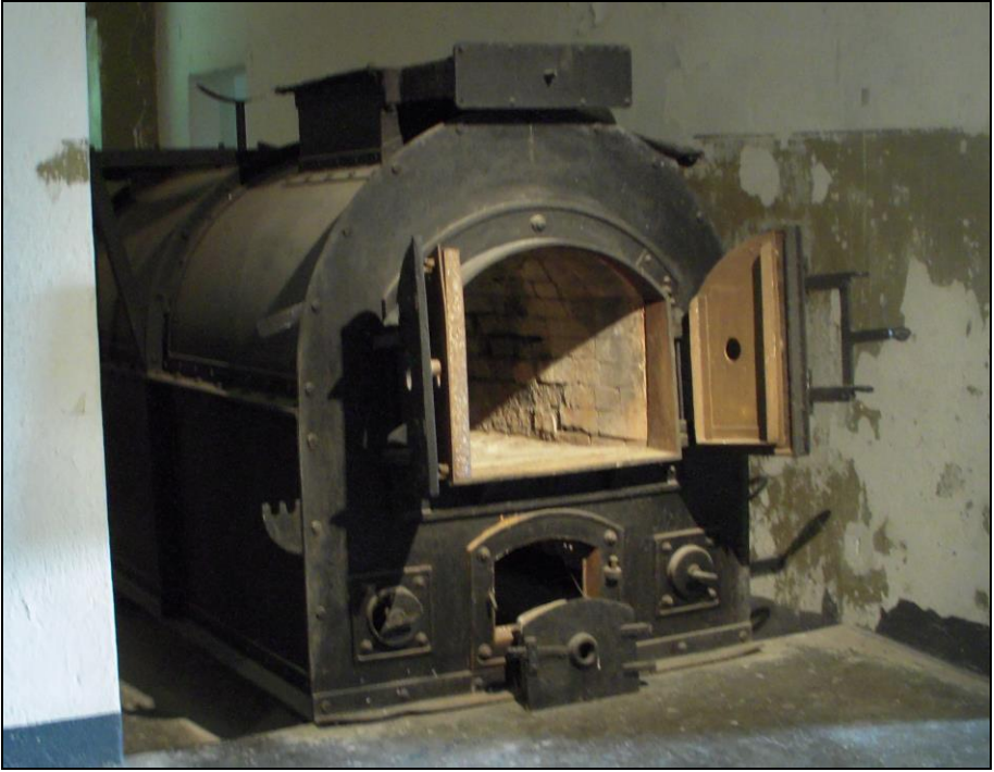
Photograph 340: KORI naphtha-fired cremation furnace at the Dora-Mittelbau Concentration Camp. Source:
