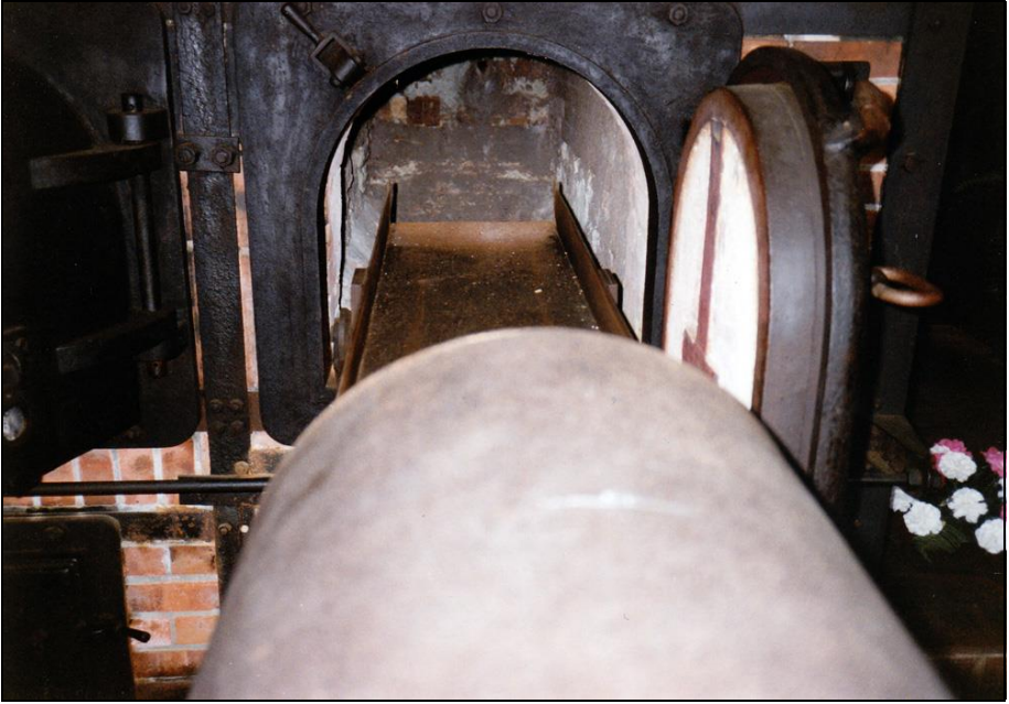
Photograph 185: view across the corpse-introduction cart with stretcher inside the muffle.
