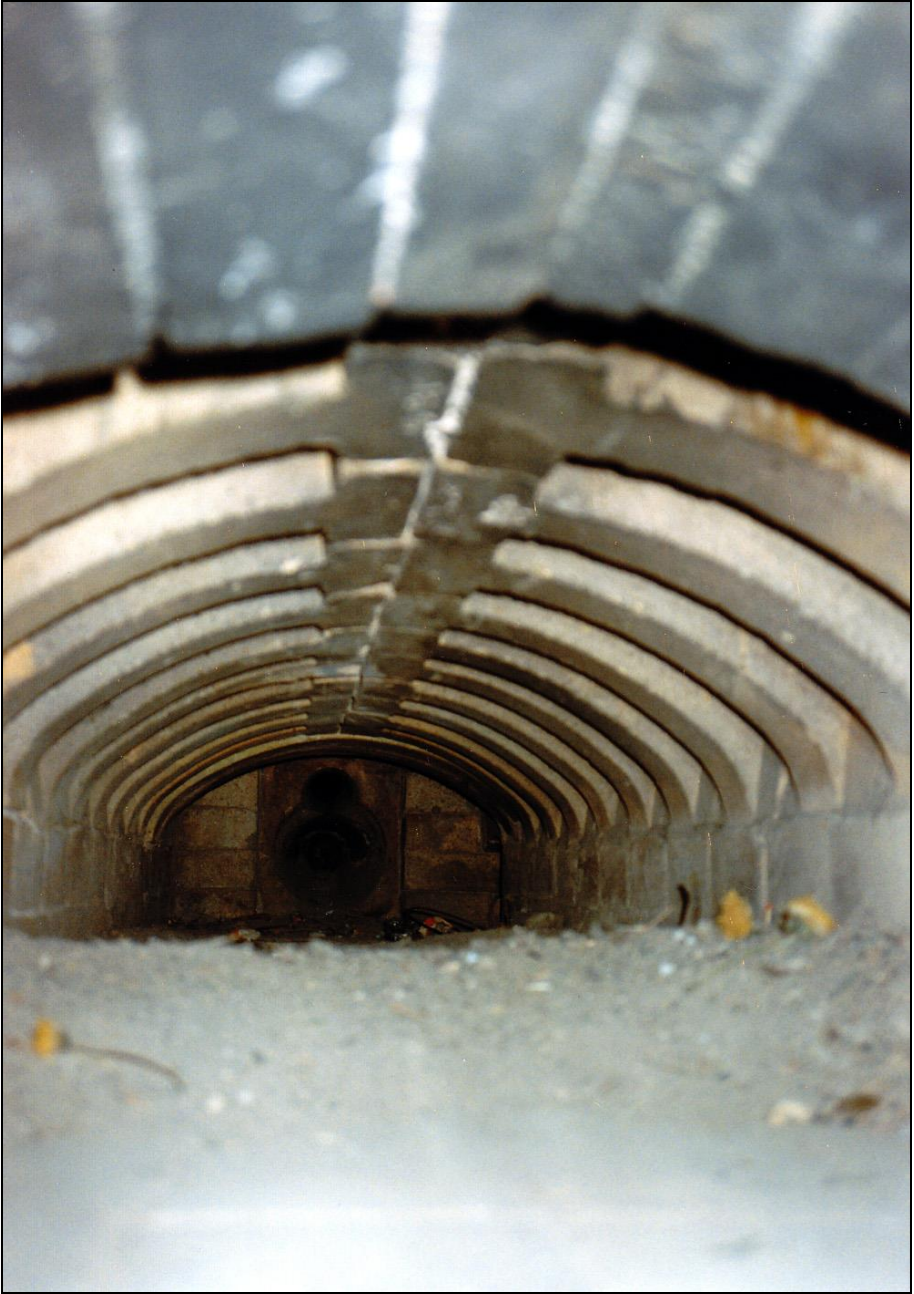
Photograph 323: Ash chamber; top: the underside of the muffle's refractory grate; background: the auxiliary burner's nozzle.
